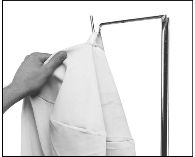
Figure 8. Attaching filter bag.
